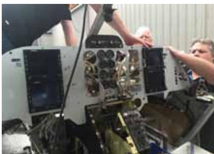
*Below left: A prototype instrument panel is installed and will become the holding fixture during the production of the wiring looms.*
