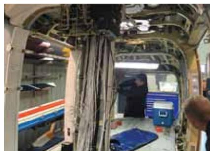
*Below right: New looms are installed in the rear cabin for an improved lighting system.*
